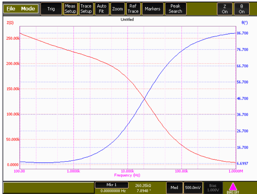
Fig. 4. Frequency characteristics of sample S_400 at RH = 97\% and a temperature of 25°C
