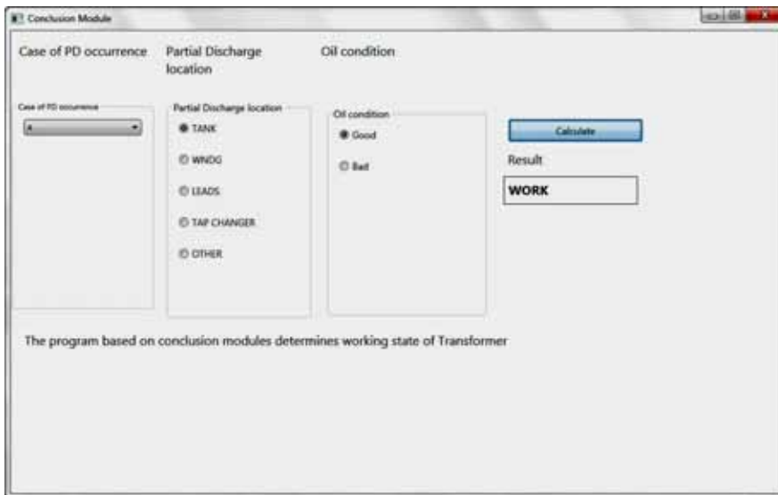
Fig. 2. Conclusion Module– case A (work state-tank)
