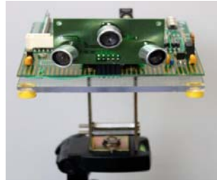
Fig. 1. The placement of the transducers in the bioinspired ultrasonic system
